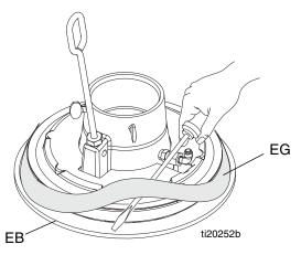
FIG. 13: Installing Spacer
